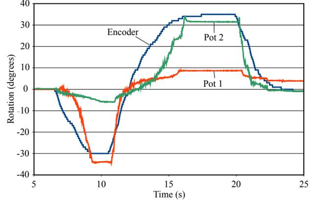
Fig. 2. Link position with 2 N driving load.  $k = 403$  N/m.
