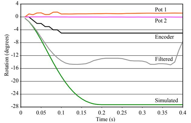
**Fig. 5.** Various measures of link position from a single run. Driving forces are  $U_1 = 1$  N and  $U_2 = 10$  N;  $k = 806$  N/m.
