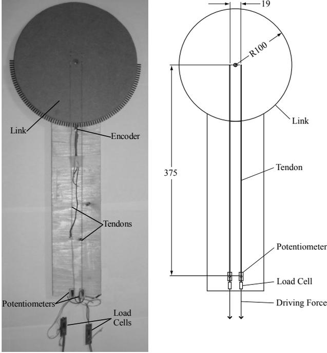
**Fig. 1.** Experimental apparatus (dimensions in mm).
