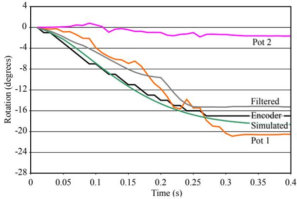
**Fig. 3.** Various measures of link position from a single run. Driving forces are  $U_1 = 2$  N and  $U_2 = 6$  N;  $k = 806$  N/m.
