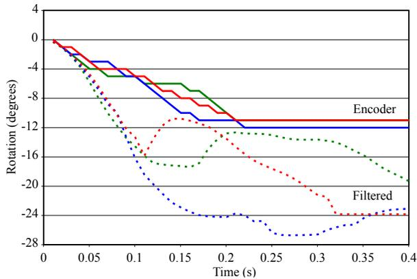
**Fig. 4.** Encoder and filtered positions over repeated runs. Driving forces are  $U_1 = 1$  N and  $U_2 = 8$  N;  $k = 806$  N/m.
